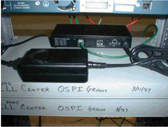
Photo 5: Close-up image of the rear panel of the Audio-Video Hub (500200). The input of the hub is connected to the audio-video source equipment.
