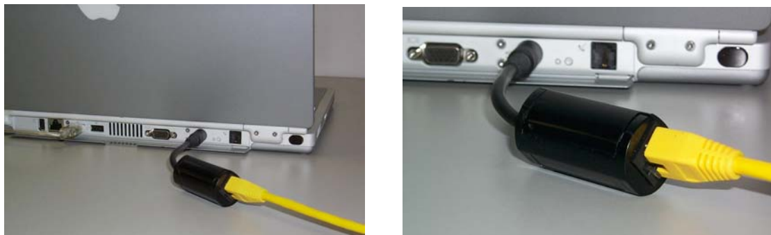
Photo 2: Close-up of S-Video Balun Connected to the Powerbook G4
