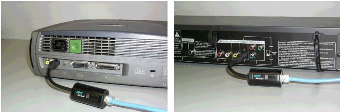
Photo 1: S-Video Balun (500016) Connected to LCD Projector and DVD Player
